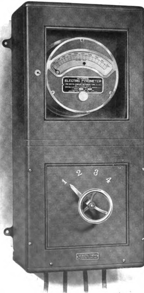
Fig. 11—Indicating instrument for electric pyrometer, with extra compartment containing rotary switch
